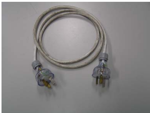
Photograph 1 extension lead with 2 male plugs
