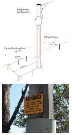
A SWER system, as the name suggests, uses the earth as the return path for the electric current. Transformers are connected between the energised line and the earth.
