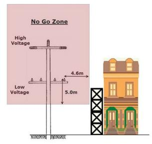
Note: For service cables guidance please refer to ESV document "Erecting, dismantling and use of scaffold near overhead service lines".
