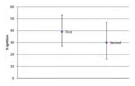
Figure 46: Difference in ignition probability with a 30 second delay
