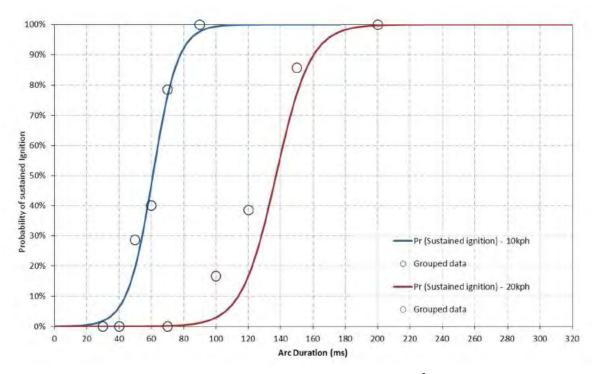
Figure 43: Effect of wind speed on Ignition probability (200 amps, 45°C, 5 per cent moisture)
