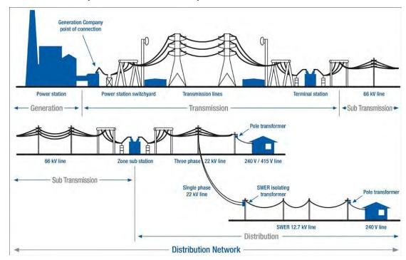
Figure 1: Schematic view of Victoria's electricity supply system<sup>28</sup>
