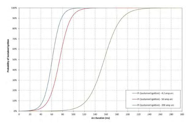
Figure 42: Ignition probability against arc duration for 4.2, 50 and 200 amp arcs at 45°C and 10 km/h wind speed for hay/straw at 5 per cent moisture
