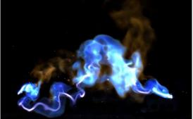
Figure 10: Electric arcs produced during testing – from the 4.2 amp testing on the left, and the 200 amp testing on the right
