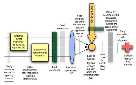
Figure 48: Code Red day electrical fire start threat-barrier diagram
