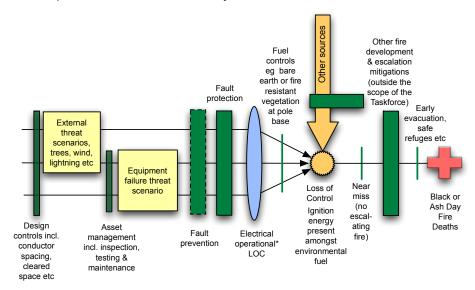
Figure 47: Fire season electrical fire start threat-barrier diagram
