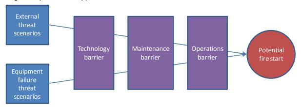
Figure 17: Threat-barrier diagram for the ignition of bushfires by powerlines on a Code Red day Figure 17 indicates that the threats arise from faults on powerlines caused by:
