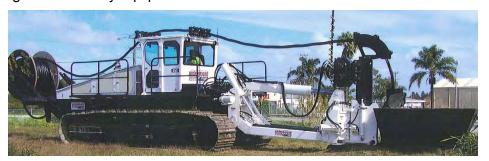
Figure 20: Plough for undergrounding cable
