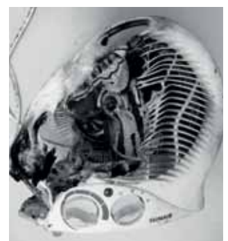
The Sunair fan heater – before it caught fire and afterwards!
