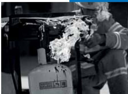
What can go wrong when the connection between a BBQ and gas cylinder becomes loose.
